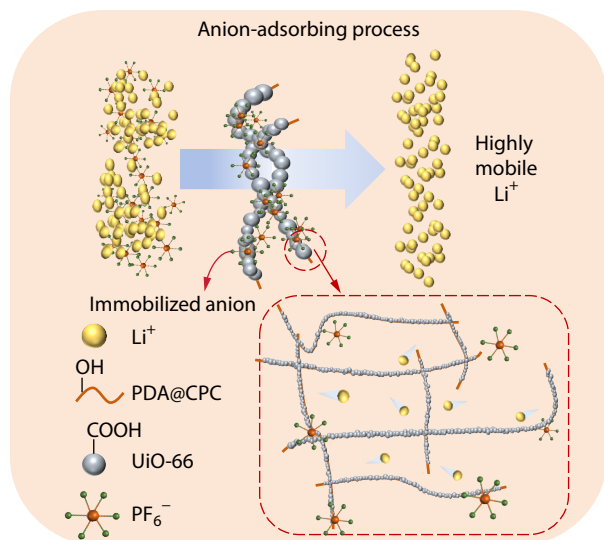
Fig. 8 Schematic diagram of ion migration in UiO66@PDA@CPC ENS assembled batteries.
